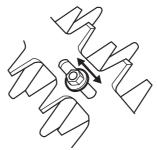
• Replace the blades if they are bent or damaged.
